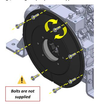
**Important Note** • To avoid axial loads that are dangerous for the engine, housing assembly on the flywheel must be carried out smoothly, without forcing it.
