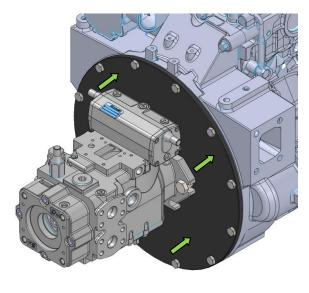
**Important note** • To avoid dangerous axial loads for the engines, housing assembly to the flywheel housing must be carried out smoothly, without forcing it.
