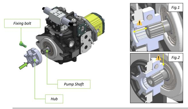
Important A Make sure that the hub doesn't touch any fixed parts of the pump (see fig.3), otherwise it is not suitable and must be replaced with another item with a different profile (see fig.4).
