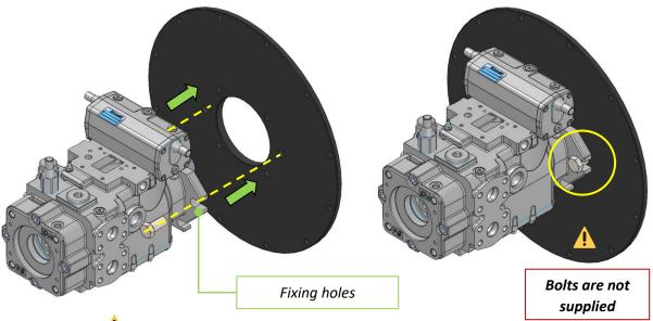
\*Important note 4 Bolts to flange, housing and pump are not supplied.
