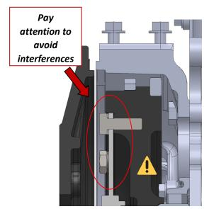
Important note • Make sure that the bolts that are used to fix the flange will not interfere with the internal surface of the housing.
