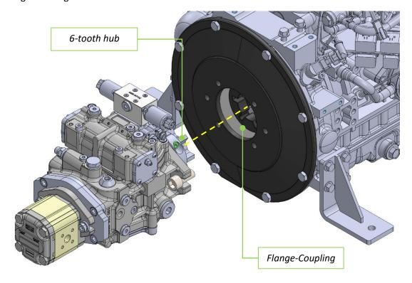
Rotate the pump to make the center of the bolts\* coincide with the pattern of the tapped holes on the housing.
