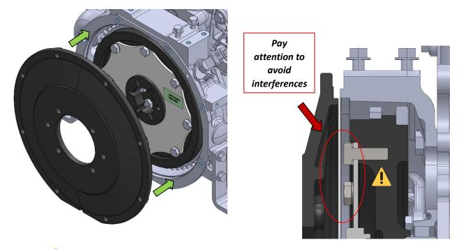
**Important** • Make sure that the bolts\* used to fix the flange do not interfere with the internal surface of the housing.
