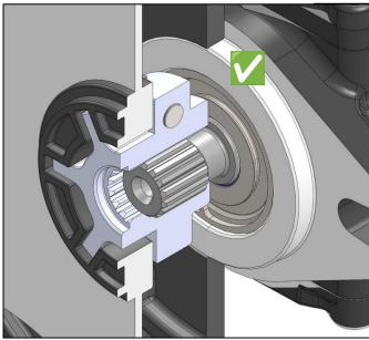
Important A Based on the relevant dimensions or the spigot, make sure that hub teething will totally fit to flange teething (see fig.5 and fig.6)
