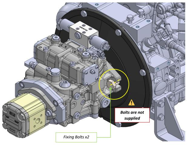
\*Important Note 1 Bolts to flange, housing and pump are not supplied.
